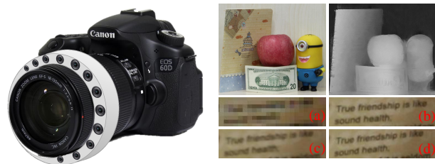
Fig. 1. Left: Conceptual design of our light field lens attachment. Right: The top left image is a scene captured using our system, and the top right image is the estimated disparity map. The bottom four images are: (a) an image patch from a side-view camera, (b) an image patch from the center-view DSLR camera, (c) the patch-based super-resolution result, and (d) the super resolution result obtained using our method.
